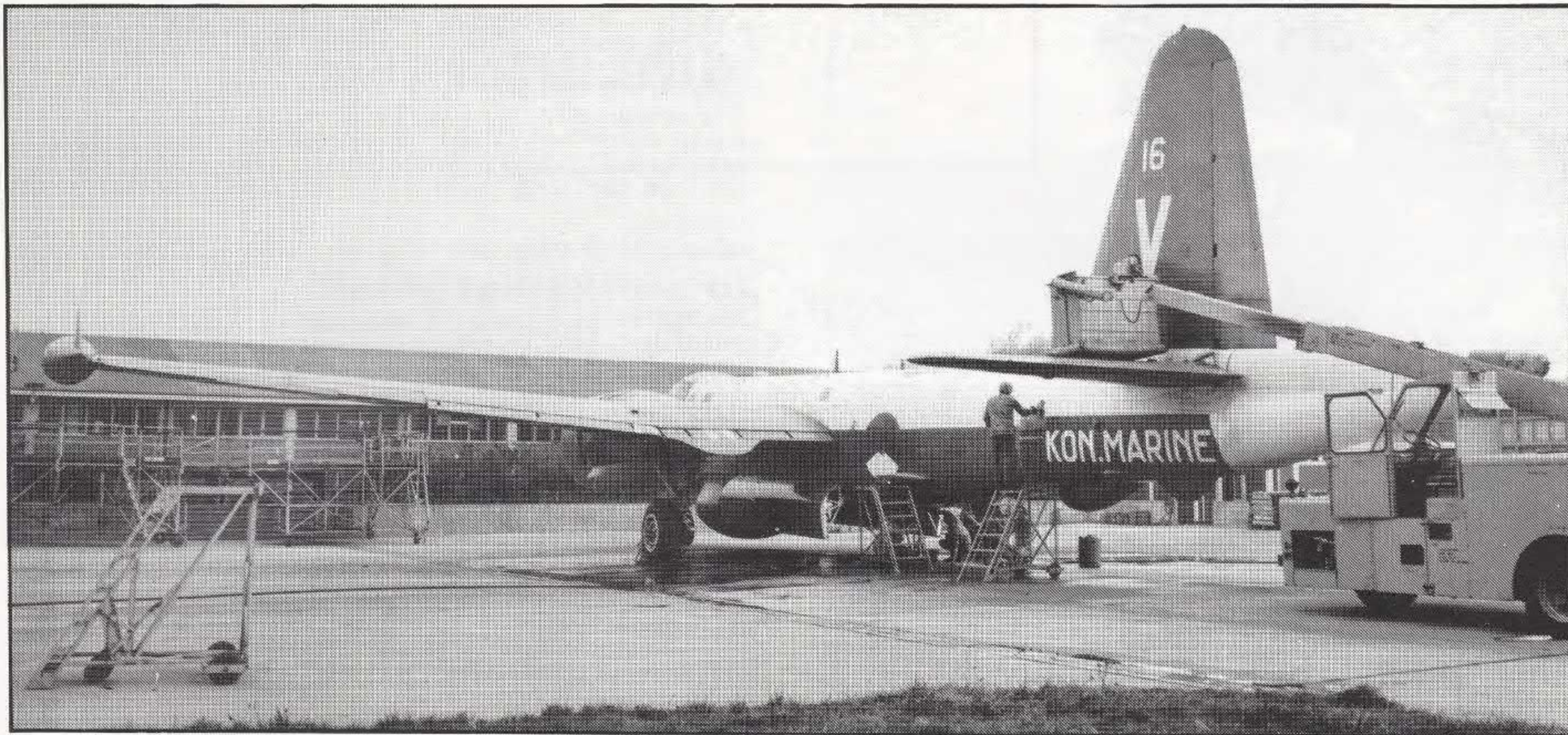
Corrosion control is essential for aircraft operating over sea. Washing the aircraft is one of the items of corrosion control.
