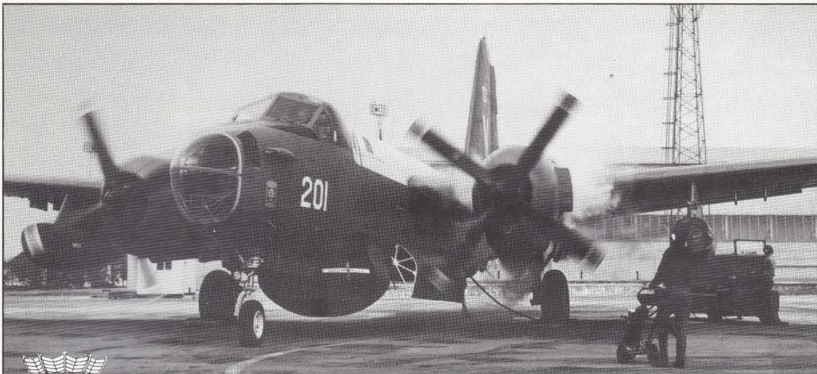
A well-known sight at Valkenburg is the smoke coming of the Pratt and Whitney R.3350-32W piston engines when being started. A well-known sight which is about to disappear. (All photos: Kon.Marine/Audio Visuele Dienst)
